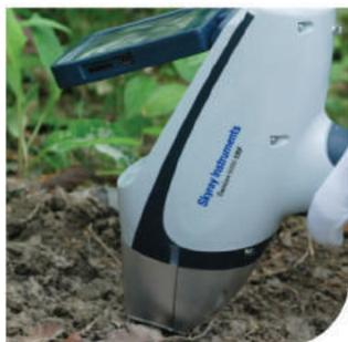
Genius Handheld XRF Spectrometer features rapid non-destructive elemental identification and composition analysis with SDD Detector for precise detection of any element from Magnesium to Uranium. Performance and accuracy similar to Desktop XRF System combined with convenience and portable size factor of a Handheld XRF. Genius XRF is suitable for wide range of applications with multiple software options to choose from.
