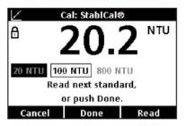
In the full calibration mode (0 to 1000 NTU), the text-based, assisted calibration feature walks you through clear and easy steps, and verifies the accuracy of your calibration automatically. This on-screen assistance eliminates the need for a manual and provides assurance that your calibration is complete and valid.
