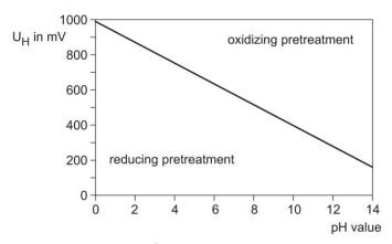
Oxidizing pretreatment Immerse the platinum electrode for two to three days in a sulfuric Clorina solution. Clorina powder for producing the solution is included in the SORT/RH reagent set.
