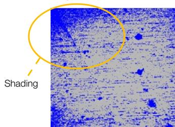
Shading correction produces even illumination across the field of view.
