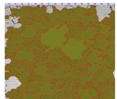
Grain sizing planimetric solution
