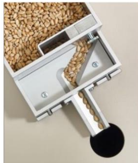
Figure 22: Flow of the seeds into the channel Start the count and observe the flow of the seeds.
