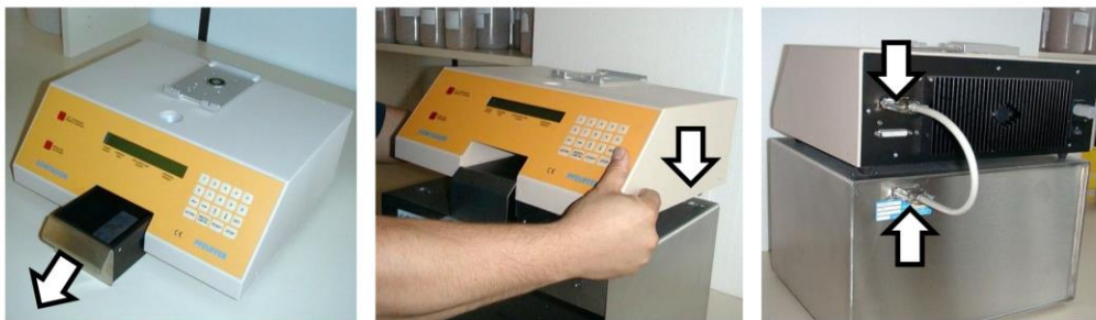
Figure 9: Put on CONTADOR and connect with CONTAFILL
